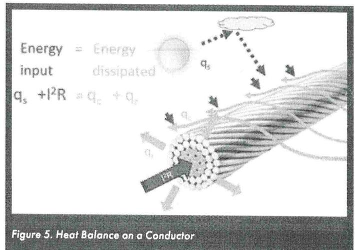
Figure 5. Heat Balance on a Conductor
