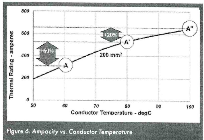
Figure 6. Ampacity vs. Conductor Temperature
