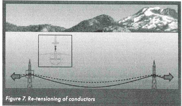
Figure 7. Re-tensioning of conductors
