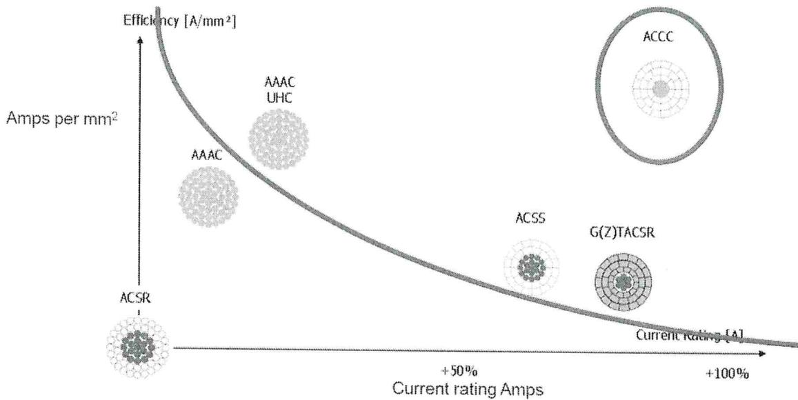
As can be seen, ACCC cables combine efficiency with increased power carrying capacity to create a clear financial advantage over other lines, and especially ACSR lines. Additionally, after a certain current threshold, ACCC cables are less expensive than the traditional ACSR cables. The table below provides the cost analysis of ACCC versus ACSR for various current requirements and conductor sizes (note, conductor sizes are represented by given names rather than precise measurements) [2]:
