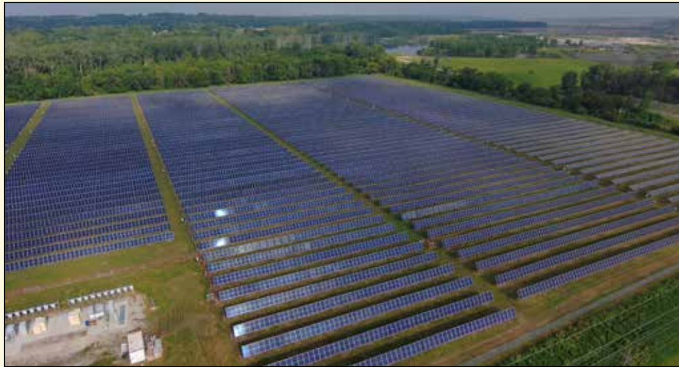
OPPD's community solar array near Fort Calhoun, Nebraska, provides 5 megawatts of renewable generation.
