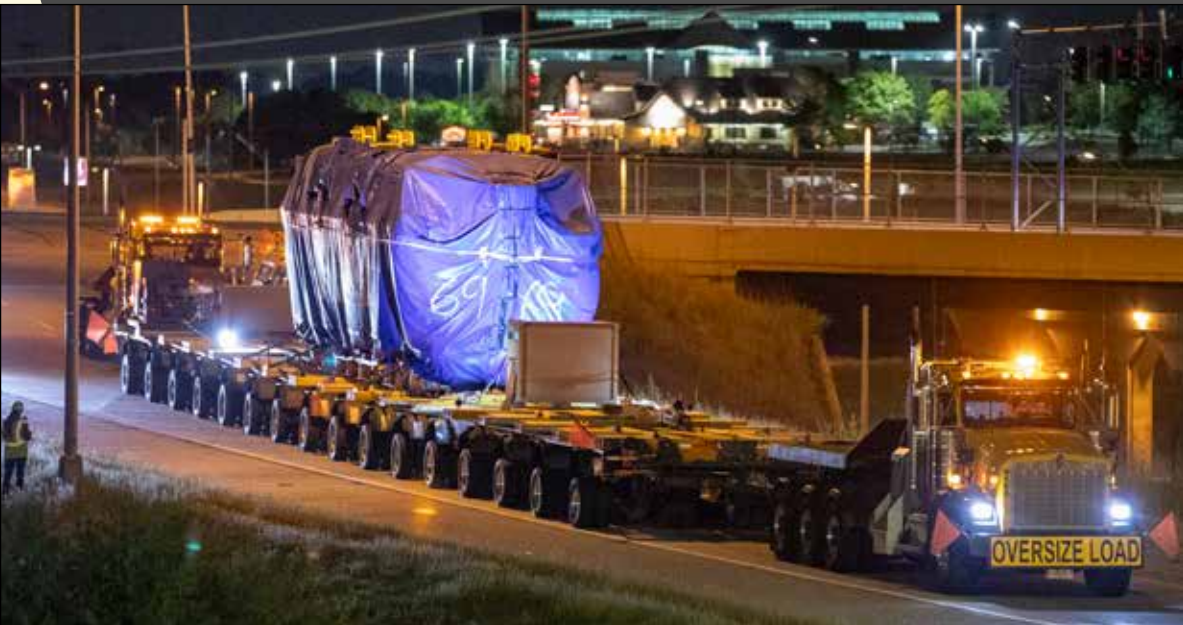
Nine reciprocating internal combustion engines were shipped to OPPD's Standing Bear Lake Station from Italy as part of the utility's Power with Purpose project.
