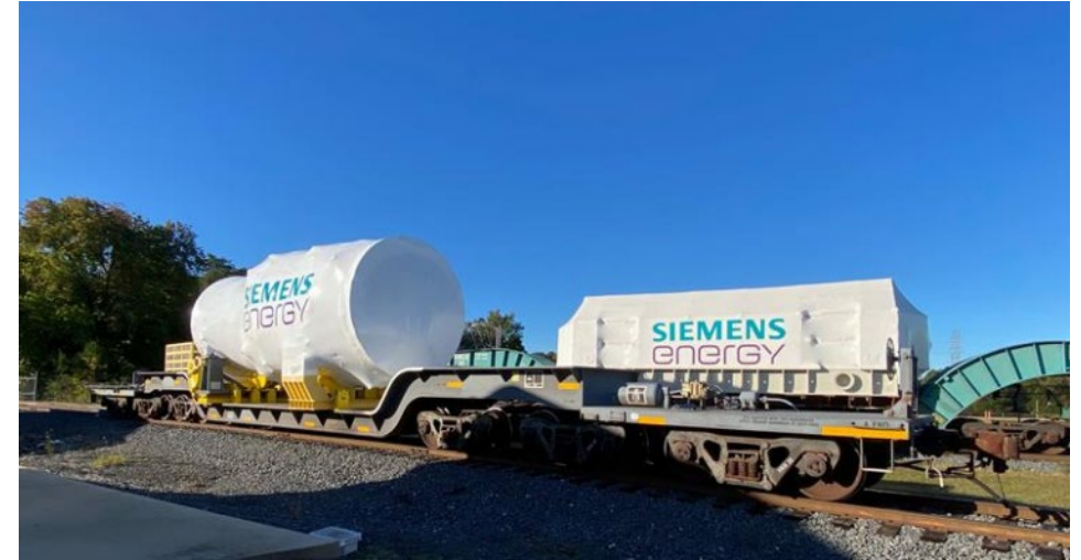
Unit 1 Siemens Combustion Turbine and Generator on rail car
