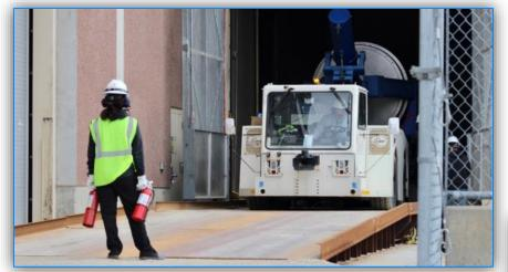
Slowly and safely, technicians transported canisters to the ISFSI and inserted them into the HSM, then securely bolted down the door
