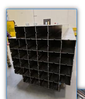
Technicians in North Carolina fabricated and welded each canister to exacting specifications, with all 944 bundles mapped to a specific location in the framework
