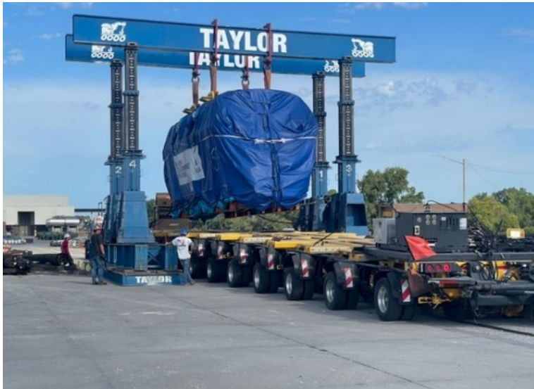
Engine being placed on trailer at ESC
