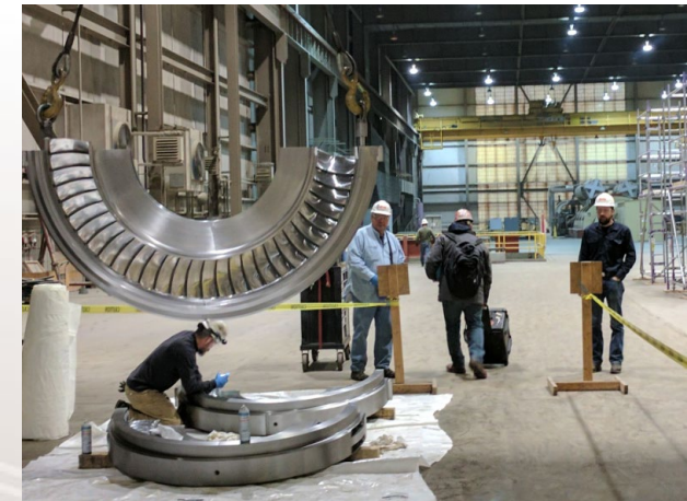
Nondestructive testing of turbine diaphragms at Nebraska City
