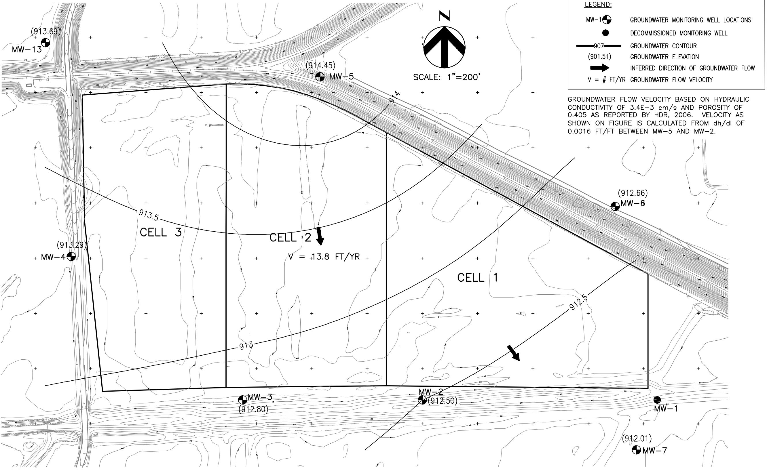
GROUNDWATER FLOW VELOCITY BASED ON HYDRAULIC CONDUCTIVITY OF  $3.4E-3$  cm/s AND POROSITY OF 0.405 AS REPORTED BY HDR, 2006. VELOCITY AS SHOWN ON FIGURE IS CALCULATED FROM  $dh/dl$  OF 0.0016 FT/FT BETWEEN MW-5 AND MW-2.
