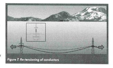
Re-tensioning may provide a moderate increase in capacity but is sometimes also required for safety code compliance and is also an appropriate technique when used in conjunction with voltage upgrading [3].
