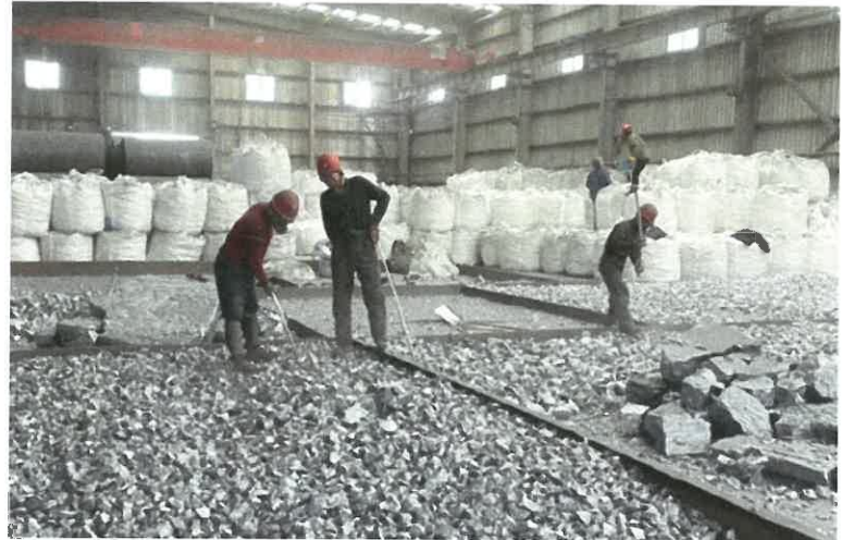
Workers manually crush silicon in Jingang Circular Economy Industrial Park, Ili Prefecture, Xinjiang. Source: Kokodala News via Weixin.
